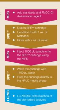
The automated sample preparation process is completed in 25 minutes. The LC-MS/MS cycle time is less than 20 min. Sample preparation and analysis are perfectly synchronized for maximum productivity and throughput using MAESTRO PrepAhead.
