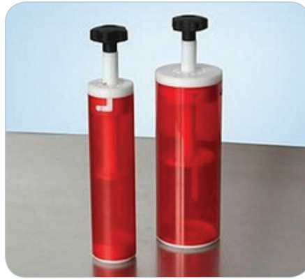
The red light inside the new restrainers is perceived by the rodents as a dark cave and therefore a safe place
