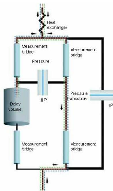
Figure 2. Schematic of the differential viscometer design.
