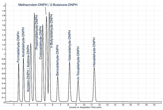
*Figure 3. Representative mass chromatogram of DNPH-derivative calibration standard.*
