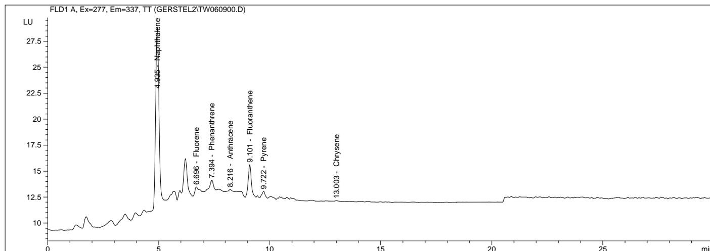
**Figure 4.** Chromatogram of a precipitation water analyzed by SBSE Twister Back-Extraction (extraction time 1 h; desorption time 8 min at 38 °C and 750 rpm; PAH concentrations determined by calibration of SBSE: naphthalene: 225 ng/l, fluorene 3.0 ng/l, phenanthrene 3.5 ng/l, anthracene 2.5 ng/l, fluoranthene 10 ng/l, pyrene 5.6 ng/l, chrysene 2.3 ng/l).
