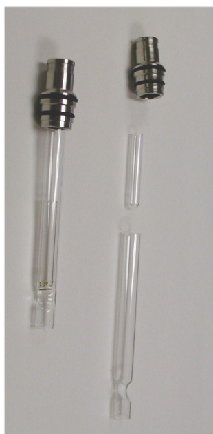
Figure 1. TDU empty tube with microvial.
