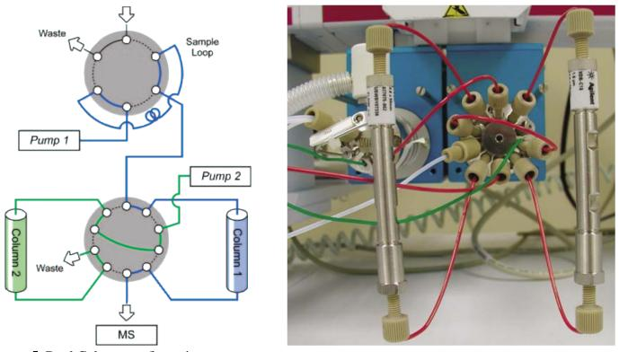
Figure 5. Dual Column configuration.
