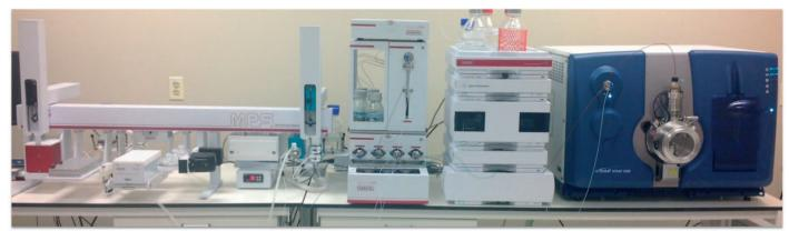
Figure 2. GERSTEL MPS XL with SPE<sup>XOS</sup> coupled to a QTRAP<sup>®</sup> 4500 system.
