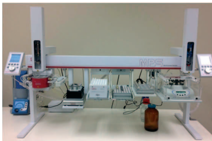
Figure 1. GERSTEL MultiPurpose Sampler (MPS XL) configured for automated extraction of mycotoxins from food samples.
