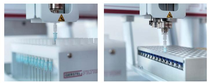
Figure 3. Pictures of the MPS transporting the 0.45  $\mu$ m filter from the filtration tray (left) to the VT-98 tray with filtration cover (right).
