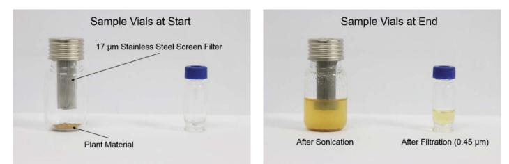
Figure 4. Sample vials at the start (left) and end (right) of the automated sample preparation protocol.
