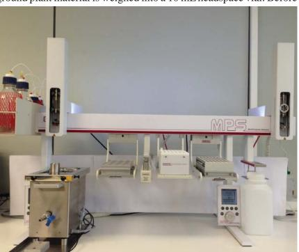
**Figure 1.** MPS Dual Head WorkStation configured for automated ultrasonic extraction and filtration.
