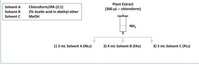
Figure 2. Automated SPE procedure.
