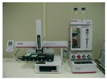
Figure 1. DBSA-SPExos-LC/MS/MS configuration.
