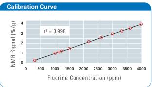
The method is calibrated with 3 to 5 samples of known fluorine content. Aqueous NaF solutions are recommended as calibration samples. Alternatively, solutions of other APIs may be used. The weight-normalized NMR signals (amplitudes) are correlated with the fluorine content by linear regression.
