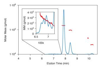
The power of UHPLC for separating aggregates and fragments combines with MALS to unequivocally identify small quantities of impurities in an IgG sample. Each of the aggregate peaks shown in the 100x inset represent a fraction of one percent of the monomer total mass yet is well-quantified by MALS.
