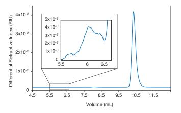
While Optilab and microOptilab offer the same sensitivity as the top industry dRI detectors for HPLC and UHPLC, no other can match its dynamic range. This chromatogram of galactose shows just a portion of the full range. The impurity shown in the inset, validated across five replicates with perfect repeatability, has been magnified by >100,000x relative to the primary sugar peak.
