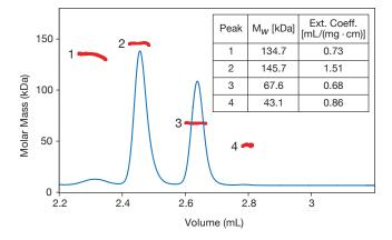
Absolute molar mass is determined from light scattering intensity and concentration, without reference to column calibration or assumptions regarding conformation and non-ideal column interactions. Optilab is perfectly matched to Wyatt Technology's MALS detectors, making dRI measurements at the same wavelength as the MALS laser.
