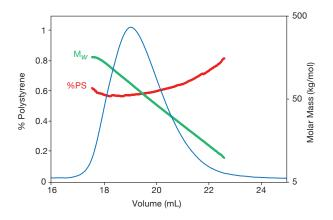
The triple-detector combination of MALS, dRI and UV is essential in characterizing conjugated complexes such as glycoproteins or copolymers for which no reliable column calibration standards exist. Here poly(styrene-co-acrylic acid) is analyzed to determine both total molar mass and percent polystyrene across the entire peak.
