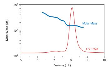
The miniDAWN is a perfect MALS detector for size-exclusion chromatography (SEC) in order to determine absolute molar masses and sizes of proteins or polymers eluting from the SEC column (IgG and oligomers shown here as an example). Its superior solvent compatibility and minimal maintenance requirement make it a robust tool for SEC-MALS. Furthermore, it can be augmented with an online DLS option and/or the ViscoStar<sup>®</sup> viscometer.
