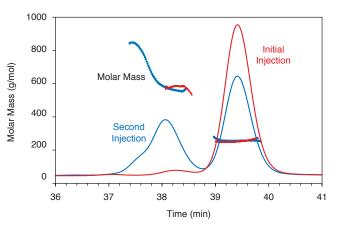
Methylene diphenyl 4,4'-diisocyanate (MDI) has a molar mass of 250 Da and will readily form oligomers in THF. The superior sensitivity of the miniDAWN permits accurate characterization of low molar mass molecules like MDI, without reference to standards or column calibration of any kind. Over time, the sample aggregated and shows more oligomers (blue curve) compared to the initial injection (red curve).
