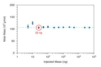
The miniDAWN provides sensitive, precise, and accurate measurements of the molar masses (MM) of polymers as demonstrated by the graph of MM vs. Injected Mass from a  $1.05 \times 10^5$  g/mol polystyrene. The results were obtained from a 7.8 x 300 mm SEC column using THF as the mobile phase. Each data point is the average from three runs. The graph shows that accurate and precise MM is readily achieved with an injected mass of 25 ng and above.
