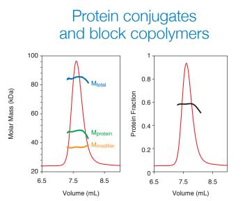
The ASTRA workspace has rich features for characterizing modified proteins using the Protein Conjugate Analysis algorithm which uses simultaneous signals from UV, RI and MALS. The characterization results includes molecular weight, protein and modifier mass fractions, extinction coefficient and composition analysis. The same analysis works or copolymers as well.
